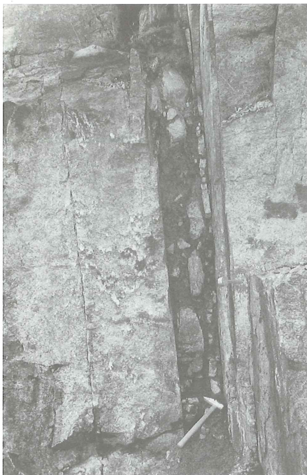
Fig. 7. Subvertical fault in granitic gneiss, Sotra. The completely non-cohesive fault rock consists of rounded fragments in a sandy matrix of similar composition as the side rock, indicating that the fault rock formed by grinding at a shallow crustal level. See Fig. 5 for location. UTM 808904.
